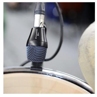
If the drum sounds too thin, it is recommended to bring the microphone close to the instrument
